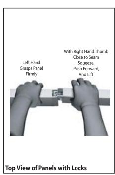
The first level of components contain pane locks that are located at the top of the panel for extra stability and seamless connection. When disassembling panels twist top connection slightly and lift right panel upward.
